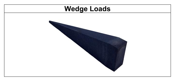
Thorndike Wedge loads come in both low and high power versions. They are typically used for semi-precision applications and higher power applications where the heat generated can be removed through the waveguide walls. These loads typically cover full waveguide bandwidths with an estimated VSWR of 1.10:1 or better. Performance at the very low end of waveguide bands may deteriorate slightly for shorter length wedge loads.
