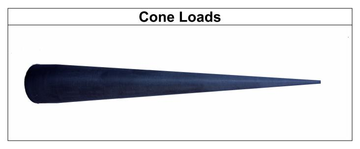
Thorndike Cone loads are precision machined, linear tapered, lossy inserts to give the best VSWR over the widest frequency range. They can be used for precision bench measurements and calibrations when the most accurate measurement results are required. They are typically used as calibration loads when making return loss or VSWR measurements using vector network analysis techniques. These are used in waveguide calibration kits to remove equipment errors during reflection measurements.
